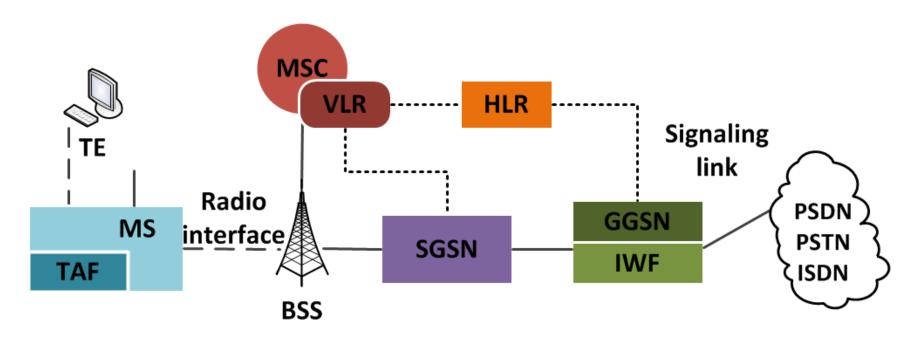
HLR : Home Location Register VLR : Visitor Location Register MSC : Mobile Switching Center MS : Mobile Station (Handset) BSS : Base Station Subsystem SGSN : Serving GPRS Support Node GGSN : Gateway GPRS Support Node TE : Terminal Equipment IWF : Interworking Functions PSTN : Public Switched Telephone Network
